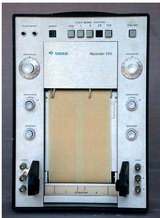
FIGURE 1-7. Mechanical recorder used to collect hemodynamics and popular in the 1980s and early 1990s.
