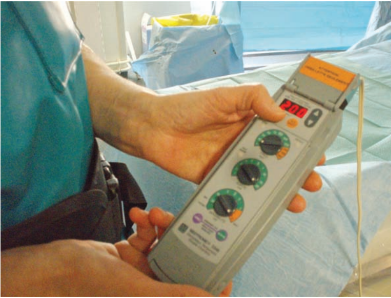
Figure 7 The Medtronic 5348 temporary pacemaker used for rapid pacing.
